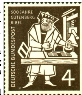
Fig. 2—Gutenberg using ink balls to ink a form of type on the bed of a press; Germany 723
